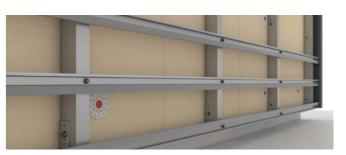
Horizontal battens must be fixed to the vertical profiles in each intersection. In areas where two consecutive horizontal battens meet, the following must be taken into consideration:
